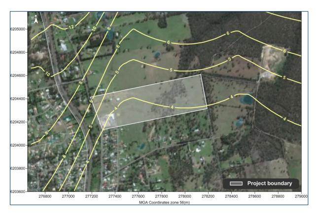
Figure 7-1: Predicted maximum 24-hour average PM<sub>10</sub> impacts due to the Tahmoor Underground Coal Mine
