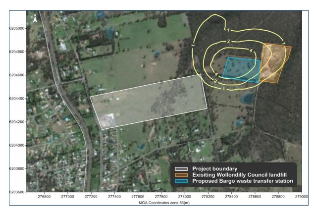
Figure 6-2: Predicted 99<sup>th</sup> percentile nose-response average ground level odour concentrations – existing Wollondilly Council landfill and proposed Bargo waste transfer station
