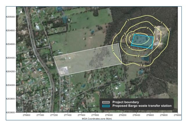
Figure 7-2: Predicted maximum 24-hour average PM<sub>10</sub> impacts due to the proposed Bargo waste transfer station
